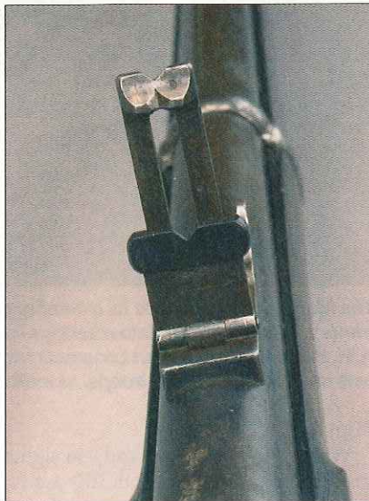
Enfield rear sights were sophisticated "ladder" affairs graduated to up to an optimistic 1,000 yards, depending upon the model and vintage of the arm.
