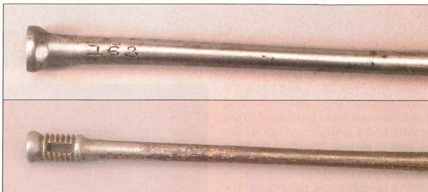
Early Enfield ramrods had simple "button-head" tips. This was later changed to a knurled, slotted end to allow better grip and more torque when using musket tools.
