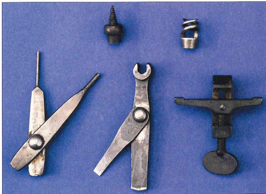
Springfield tools involved (top to bottom, left to right) bullet puller, worm, tumbler and wire punch, screwdriver/nipple wrench, mainspring vise.
