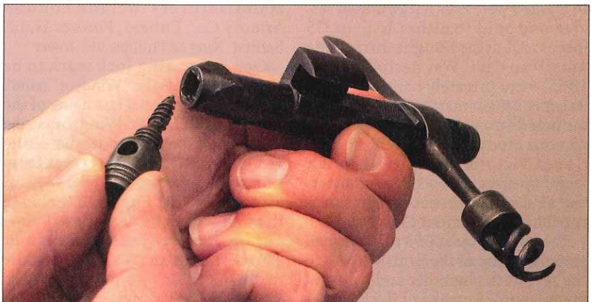
The Enfield sergeant's tool was a clever all-in-one arrangement that contained a bullet puller, vent pick, oil bottle, worm, nipple wrench, mainspring clamp and screw-driver. These were not issued to every soldier in the British army.
