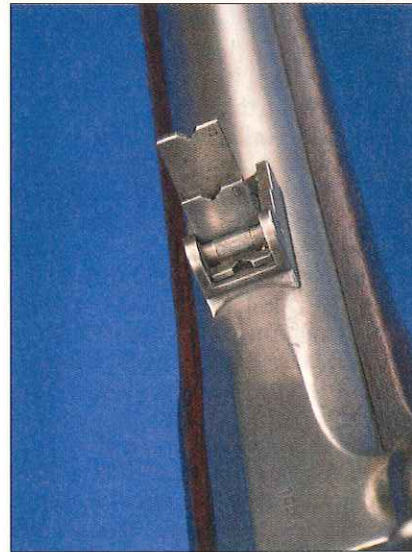
Springfield sights involved a folding two-leaf setup with notches set for 50, 100 and 300 yards. While the gun was capable of lethality at up to 1,000 yards, as might be expected most damage was done at closer ranges.
