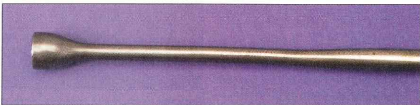
The Springfield's "tulip-head" ramrod allowed for less bullet deformation and greater ease of loading. The swell behind the head helped keep the rod in position in the stock and provided for a better grip when it was being withdrawn.
