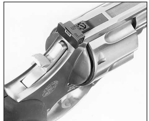
The rear sight is click-adjustable for windage and elevation and its square notch is outlined in white. A wide target-type hammer is fitted.
