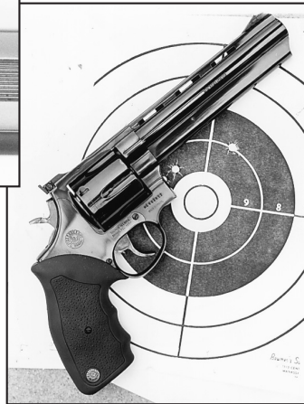
Felt recoil is reduced by a built-in compensator whose eight holes are ranged in pairs on either side of the Model 44's front sight.
