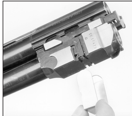
The ejectors are easily removed by pulling off the U-shaped metal strip that surrounds the monobloc. Removing the springs and plungers allows extraction-only operation.
