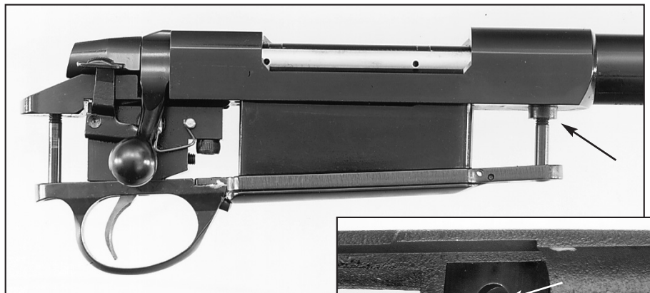
In lieu of recoil lug integral with the receiver or trapped between receiver and barrel, the Mountain Eagle uses an aluminum platform glued into the stock (arrow) that contacts the flat receiver bottom around the stock bolt, much like the Tikka M658 rifle.
