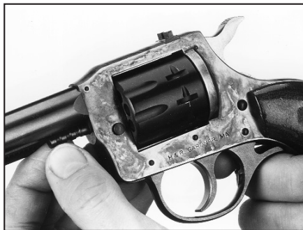
Despite the double-action trigger, the Model 949 otherwise functions like a single-action, with the expected base pin and rod ejector.
