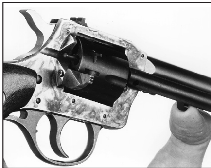
Despite the double-action trigger, the Model 949 otherwise functions like a single-action, with the expected base pin and rod ejector.
