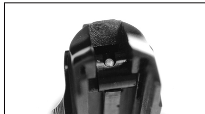
When AP22's safety lever is applied, the safety drum rotates and prevents the hammer from hitting the firing pin. In addition, the safety locks the gun's firing pin in place.
