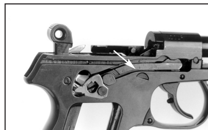
The AP22's single right-side trigger bar (above) acts on a "cocking piece." An arm on the tail of the trigger bar lifts the cocking piece, which in turn lifts the sear and cocks the AP22's hammer.
