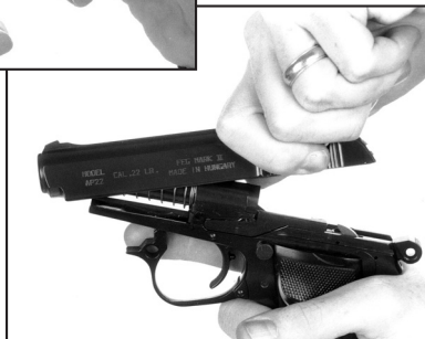
Remove the magazine from the unloaded FEG then pull down on the front of the trigger guard. Grasp the slide and pull it rearward and up—freeing it to travel forward and off. The recoil spring may then be removed.
