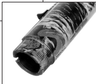
The Turkeyslayer uses an interrupted thread for barrel attachment that is further secured by the magazine nut. This type of barrel attachment is reported to be more rigid, though it makes manufacturing costs higher.
