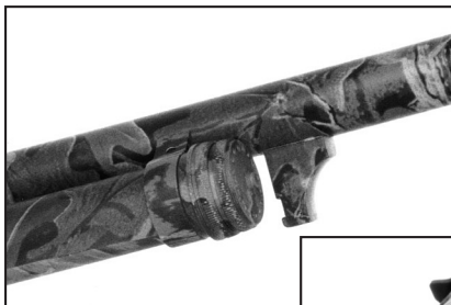
The Turkeyslayer uses an interrupted thread for barrel attachment that is further secured by the magazine nut. This type of barrel attachment is reported to be more rigid, though it makes manufacturing costs higher.
