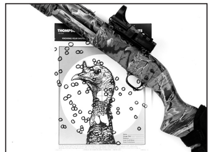
The 37 Turkeyslayer was patterned at 40 yds. with Federal Premium Magnum No. 6 shot. Patterns were tight, and easily moved to the point of aim using a C-More sight.
