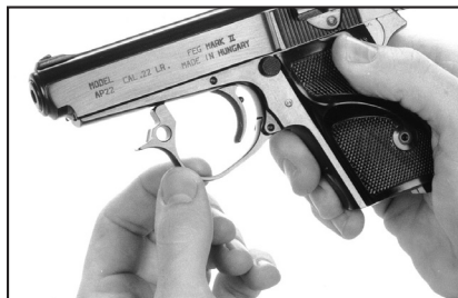
Remove the magazine from the unloaded FEG then pull down on the front of the trigger guard. Grasp the slide and pull it rearward and up—freeing it to travel forward and off. The recoil spring may then be removed.
