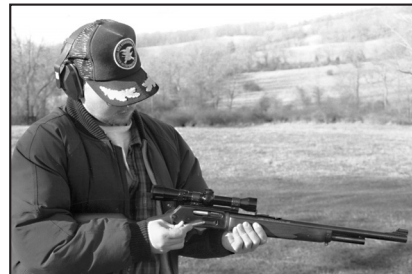
Cartridges are loaded into the Guide Gun's tubular, three-quarter-length magazine via a loading gate on the receiver's right side.
