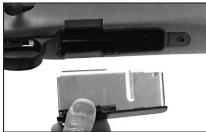
While the standard Harris Talon floorplate is steel, our sample rifle featured the optional flush-fitting Remington three-round box magazine with an alloy floorplate.
