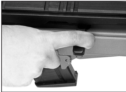
The ambidextrous bolt handle lies in line with the bore and is hinged so that it may be rotated to either the left or right side.
