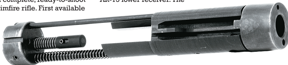
The A-22's bolt consists of a front collar that fits around the barrel extension, the bolt that rides on two guide rails, one of which is also surrounded by the recoil spring, and a steel back plate having a bolt buffer mechanism.
