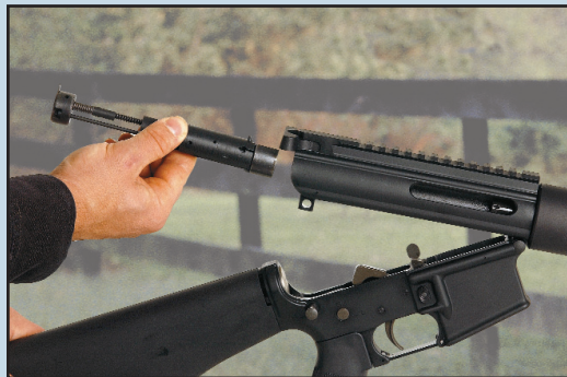
The key to the A-22 is its .22 LR blowback mechanism, which fits into the upper receiver in the same manner as a regular AR-15 bolt and carrier (r.). The A-22's recessed bolt face has twin claw extractors (below r.). The A-22 uses a 10-round .22 LR magazine made by Colt (below). A steel finger serves as the ejector. Note that there is no forward bolt assist on the A-22 receiver (below).
