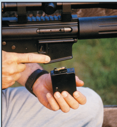
The key to the A-22 is its .22 LR blowback mechanism, which fits into the upper receiver in the same manner as a regular AR-15 bolt and carrier (r.). The A-22's recessed bolt face has twin claw extractors (below r.). The A-22 uses a 10-round .22 LR magazine made by Colt (below). A steel finger serves as the ejector. Note that there is no forward bolt assist on the A-22 receiver (below).
