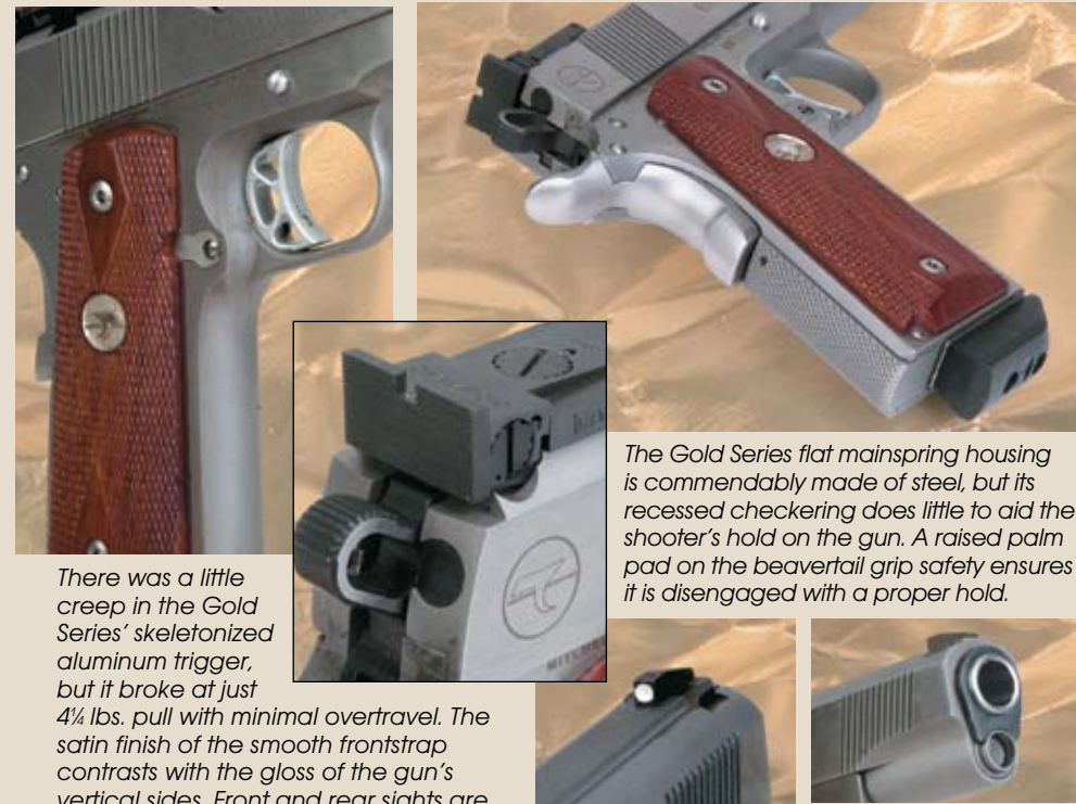
The front of the barrel is fitted to the slide with a bushing in the manner of the original government-issue 1911. The Gold series is appropriate for many types of competition because many pistol sports require this type of construction.
