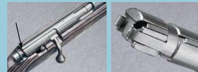
A two-position safety locks the trigger but allows bolt manipulation, while a red dot (arrow) on the cocking piece is visible when the bolt is cocked. Note grooves and tapped holes in receiver top for scope mounting. The bolt head features a non-rotating spring steel extractor and a spring-loaded inertial firing pin (above).
