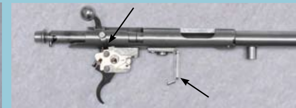
The heart of the Marlin 917VS is its cylindrical stainless steel receiver. Note safety piece attached to trigger housing (left arrow), and magazine mounting bracket and release button (right arrow).
