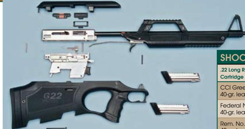
The G22 can be thoroughly disassembled for cleaning and maintenance, although the procedure is a bit complicated. Although only 28.4" long, its bullpup design incorporates a 20" barrel.
