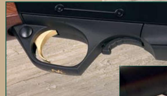
The trigger assembly (above), is contained in a polymer housing that may be removed by driving out a pair of pins, much like with many semi-automatic shotguns. The safety is a trigger-blocking crossbolt at the rear of the trigger guard. Like the lines of the fore-end, the shape of the trigger guard is futuristic.
