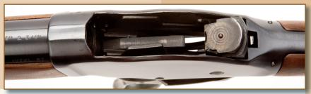
The hammer is shown fully cocked with the bolt closed (upper I.). Pulling downward on the 1887's operating lever pulls the bolt down and to the rear, (upper r.) to reveal the lifter (above).
