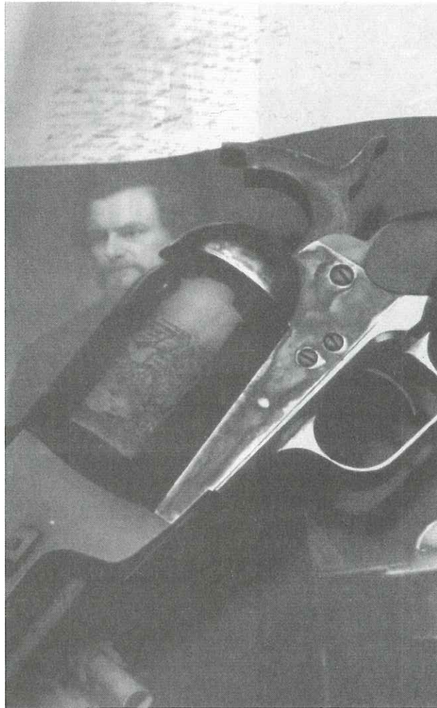
Expressly requested in 1847 by the U.S. Ordnance Department, the frame's casehardening would remain a basic characteristic for Colt military revolvers until the turn of the century.
