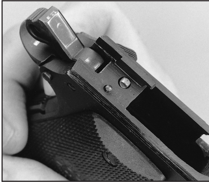
The plunger at the right of the disconnect actuates the Swartz safety system that allows the firing pin to move forward only when the grip safety is fully depressed.
