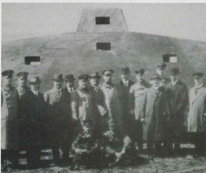
A wooden shell was fashioned over the chassis of the A7V to provide a working prototype for the A7V committee to evaluate. At one point in its development, the A7V committee was able to demonstrate the tank before Kaiser Wilhelm II and the German General Staff which had planned to use the tank as its secret weapon in the spring offensive of 1918.
