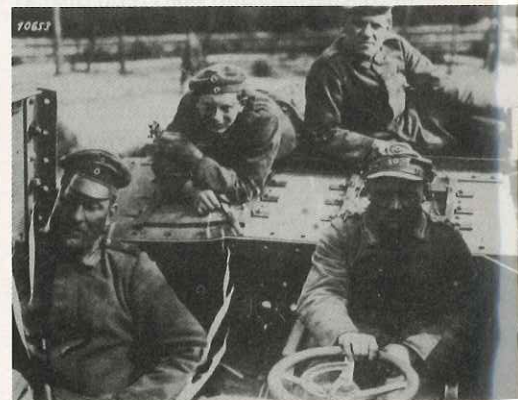
The officers and drivers of Wotan examine the driver's cupola. The sides of the cupola could be dismantled and broken down to lay flat enabling the tank to clear low overhead bridges when transported by train.
