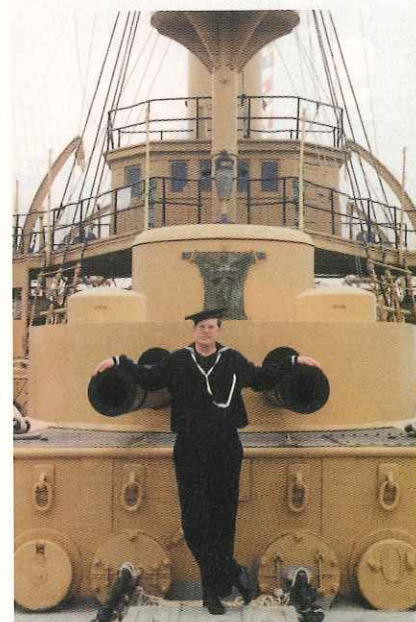
Crewman Peter Tuttle on the forward 8-inch twin turret guns. The original guns were removed and the current guns are hollow cast replicas.
